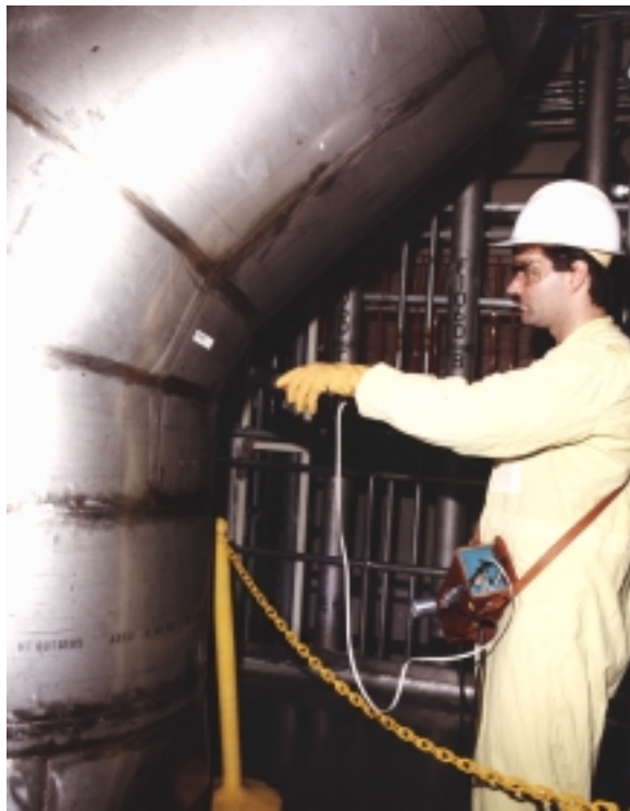
(a) Fig. 1(a) and (b). Photographs of a user performing holdup measurements on (a) a large-diameter duct and (b) a narrow pipe with the integrated holdup measurement system hardware. In both (a) and (b), the M 3 CA is in a leather pouch hanging from the shoulder of the user, the compact NaI detector is held in the user's left hand and the portable controller/data logger with bar-code reader [different models are shown in (a) and (b)] is in (strapped to the wrist of) the user's right hand. In (a), the operator is scanning the bar code on the label attached to the large duct. In (b), the operator is performing a count with the collimated detector aimed at the holdup deposit marked by the bar code on the narrow vertical pipe.
